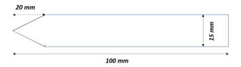
Pixi in its most basic form, write with an Edding 8300 or similar marker.
